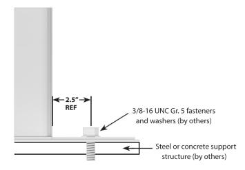
In order to avoid structural resonance, the structure must be designed with adequate stiffness so the natural frequencies are at least 120% above fan maximum operating speed.
